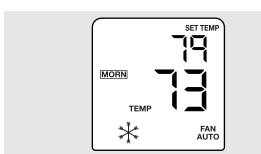
In *NORMAL* mode, press  $\blacktriangle$  or  $\blacktriangledown$ . The clock and the day of the week indicator will be cleared. The setpoint temperature and **SET TEMP** indicator will be displayed. The **HEAT**, **COOL** or **AUTO** indicator will turn on indicating the current operating system.
